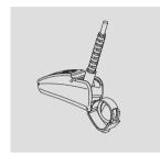
2. Plug the programming plug into the socket. Use the programming cable CS-44 A (Phonak version) only.
